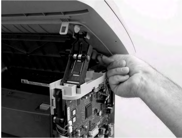
Figure 5-81. Remove the scanner assembly (7 of 13)
