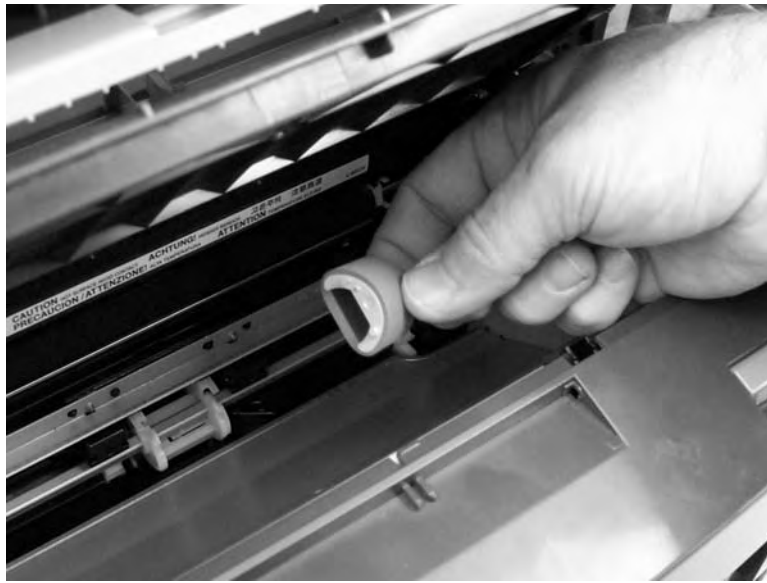
Figure 5-95. Remove the printer pickup roller (3 of 5)
