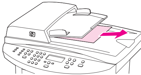
Figure 6-7. Clearing output bin jams (HP LaserJet 3020 and 3030)
