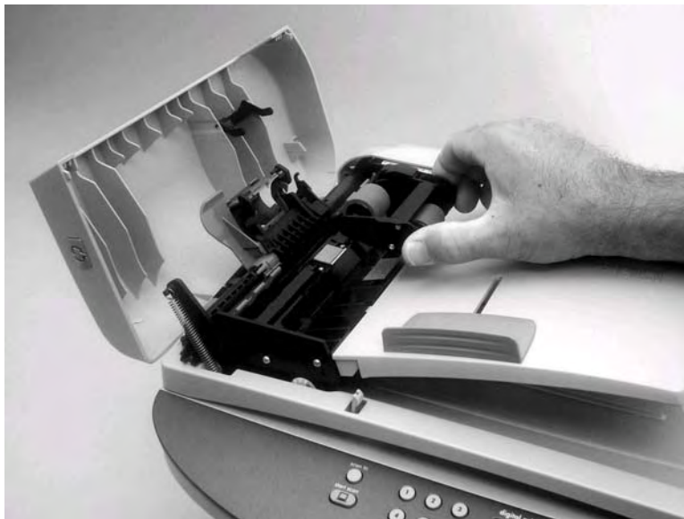
Figure 5-70. Remove the ADF pickup roller (2 of 2)
