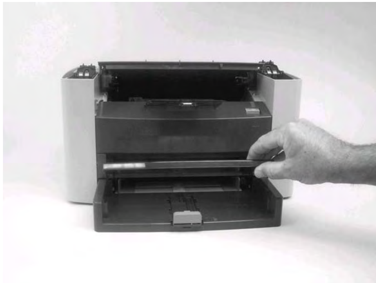
Figure 5-98. Remove the media input tray (1 of 3)
