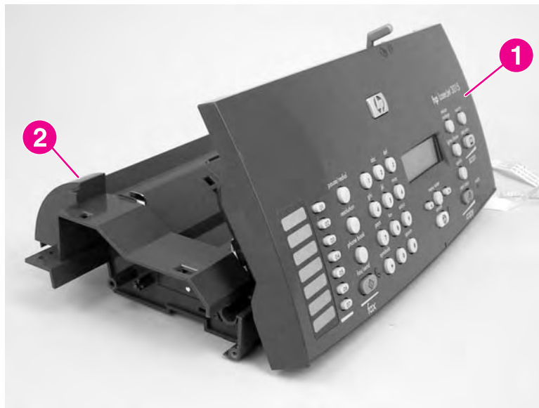
Figure 5-45. Remove the top-cover assembly (1 of 2)
