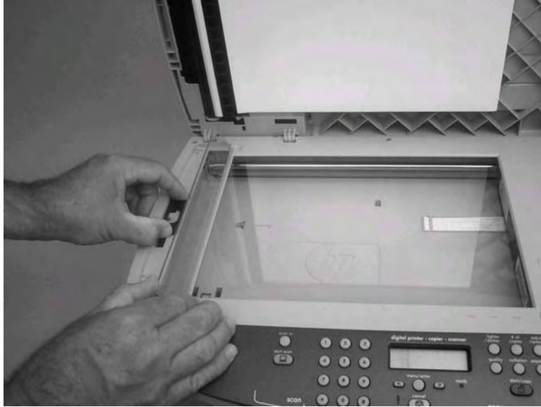
Figure 5-73. Remove the ADF scanner glass (3 of 3)
