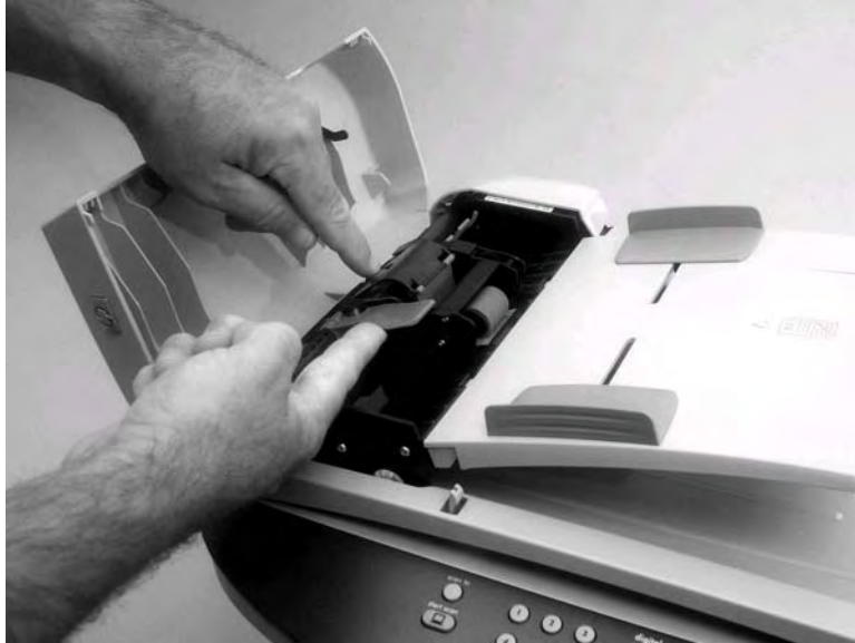
Figure 5-69. Remove the ADF pickup roller (1 of 2)
