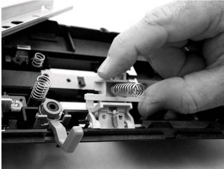
Figure 5-22. Remove the separation pad assembly (2 of 3)
