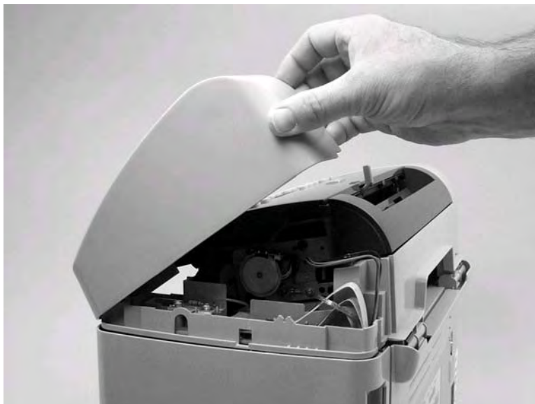
Figure 5-12. Remove the scanner side covers (3 of 3)
