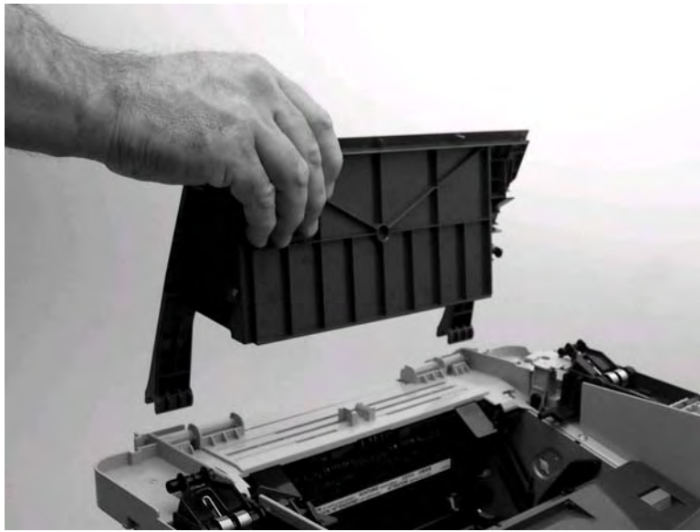
Figure 5-109. Remove the print-cartridge door (2 of 2)
