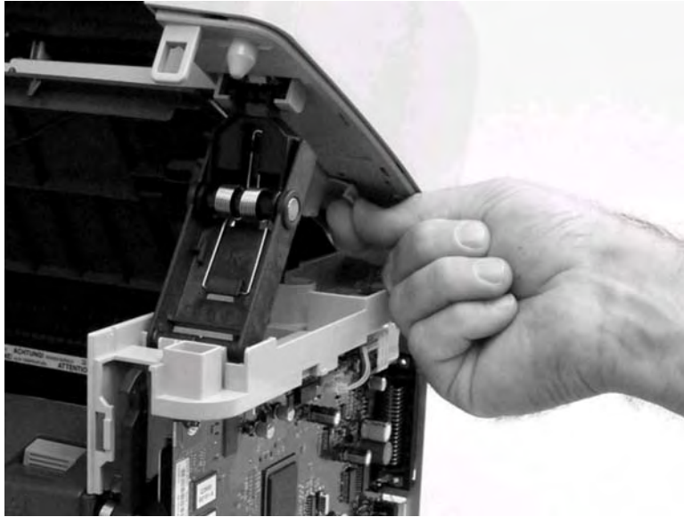
Figure 5-32. Remove the scanner assembly (9 of 15)
