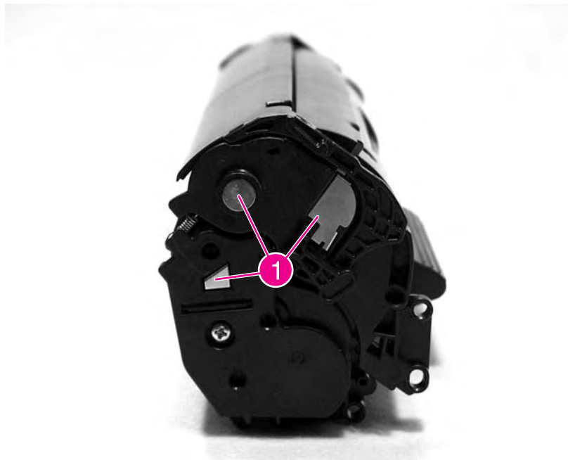
Figure 6-15. Print-cartridge high-voltage contacts
