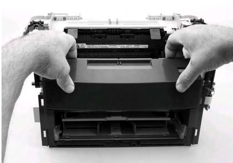
Figure 5-115. Remove the front cover (3 of 3)
